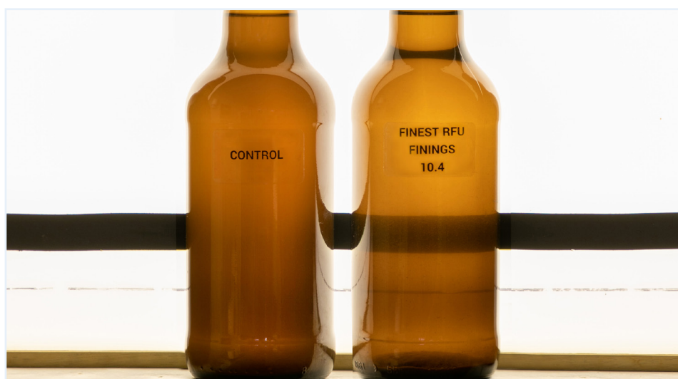
Finest RFU 0 = control, unfined beer (left). Finest RFU (10.4 ml/l): beer fined with Finest RFU (right)
