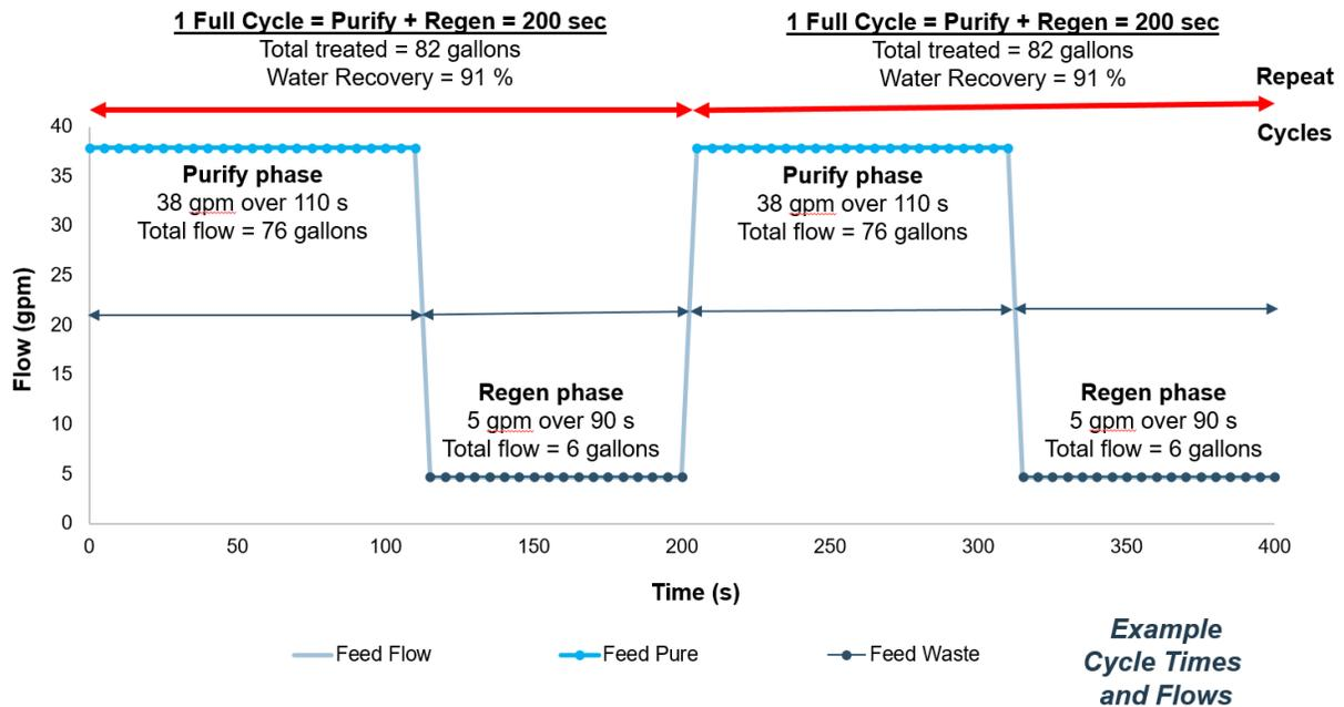
In the above flow diagram example, it is shown that the peak flow is 38 gpm and the net pure flow rate is 22.8 gpm. The net pure is lower than peak as it is averaged over the total cycle time, accounting for time when the system is in regeneration and not producing purified water.
