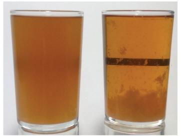
Control vs. 25ppm after 3 hours shows application of Murphy's Kettle Finings greatly increases sedimentation of cold break in wort.
