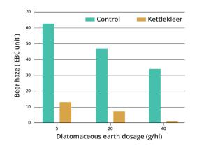
Trials show that the application of carrageenan requires less filter mateiral to produce a brighter beer.
