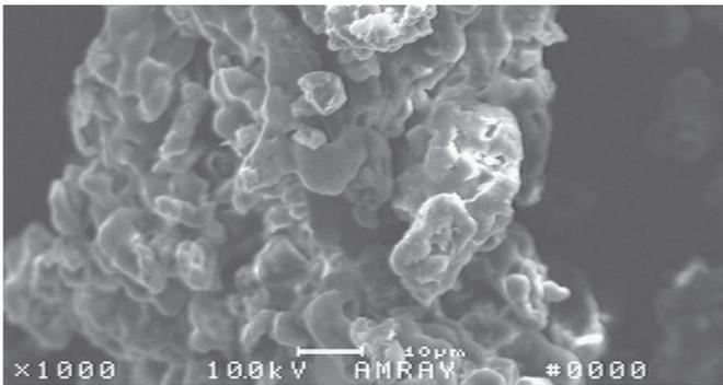
Polyclar Super R regeneration-grade beer stabilizer has a very large surface area for polyphenol adsorption making it an effective stabilizer.
